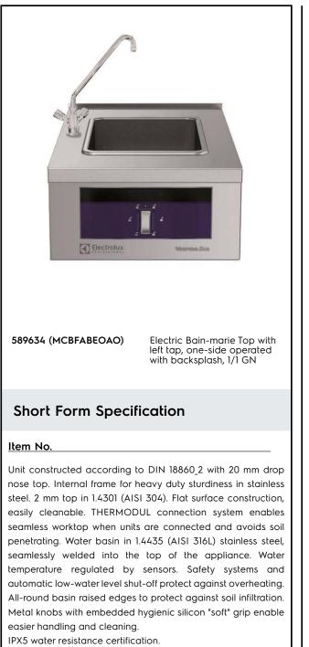
Configuration: One-side operated top with backsplash and left mixing tap.
